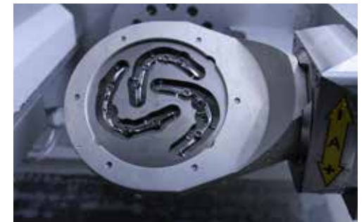
Milling a titanium frame
